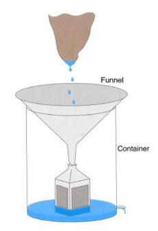
Figure 1. Drip filtration unit. The sampling container is about 10 cm in diameter and 30 cm in height. The mesh screens on the sides of the filtration bottle allow water through and retain all organisms entering via the drips.
